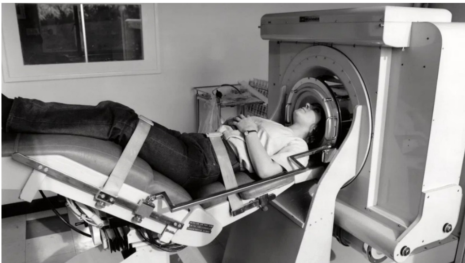
Fig. 1. The first computed tomograph (1972). Source: https://www.medmuseum.siemens-healthineers.com/en/stories-from-the-museum/history-of-ct
