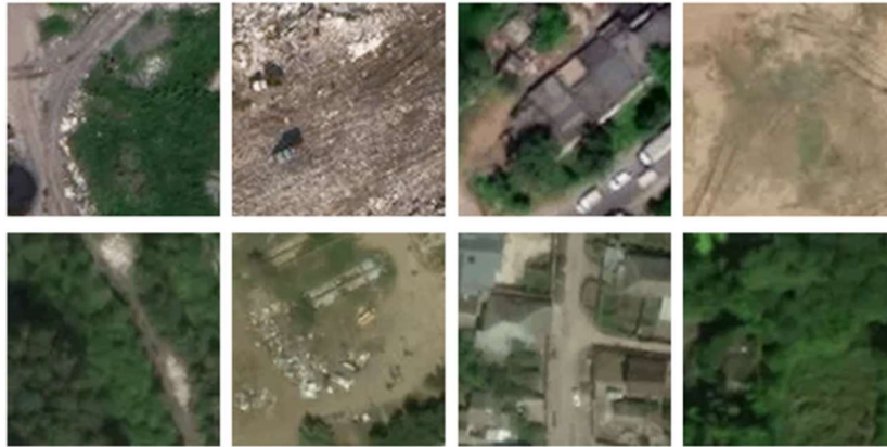
Figure 3. Images from the training set for the classification problem. The two columns on the left are fly-tips and on the right are examples of images without fly-tips.
