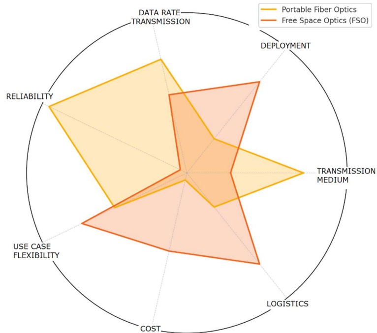
Figure 6. Comparison of portable FO and FSO in medical emergency. Source: Authors' elaboration
