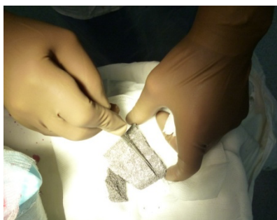
Fig. 1. Scalpel treatment of the HPCC material. The cellular structure of carbon facilitates its processing and promotes the integration of osteons into hollow cells. The volume of voids in the material reaches 90%
