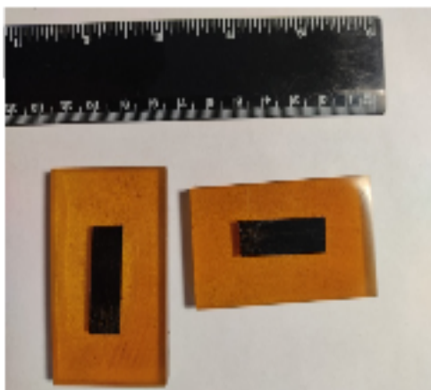
Fig.1 Samples prepared for SEM-EDS and IR spectrometry. Source: [2].
