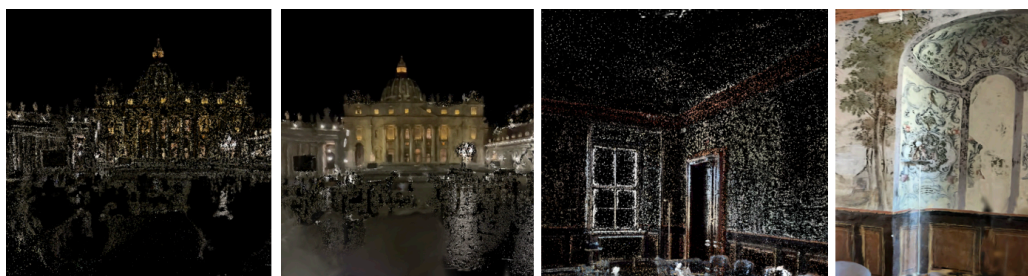
Fig. 4. An example of the process of rapid 3D documentation using an iPhone 13 PRO mobile phone (with LiDAR technology) and the Luma app. From left: a point cloud gradually forming a 3D model of Vatican Square. Next, a cloud of points gradually forms a 3D model of the Abbey Hall in the Broumov Monastery. This was not the creation of the final model. Pictures are from the authors' archive.
