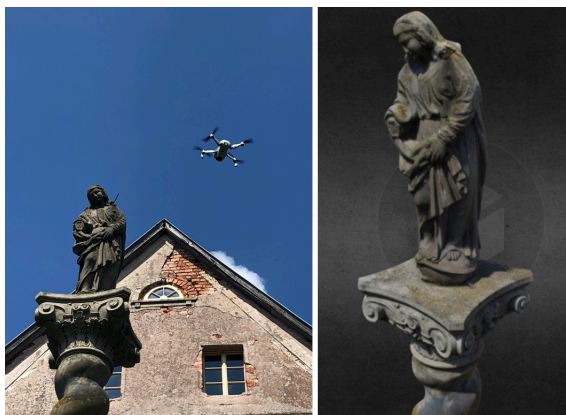
Fig. 2. Left photo of a UAV overflight. The photograph was taken during the digitization process by members of the Center for Digital Historical Sciences. The drone flying over the column with the statue of the Virgin Mary was flown by student Daniel Beneš. On the right is a sample of part of the finished 3D model. Source: Pictures are from the authors' archive, [42].
