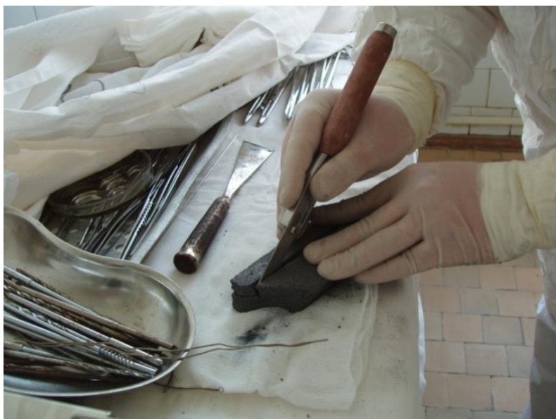
Fig. 1. Processing of highly porous cellular carbon with a scalpel. Source: authors'elaboration.
