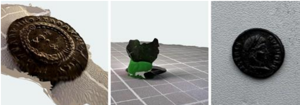
Fig. 3. These are antique coins digitized by the iPhone 13 PRO using the basic version of the Trnio program. The coin on the left has a relatively nice legible structure, but it is not sharp around the edges. In the middle of the coin embedded in the shaft- a complete failure, the smartphone did not pick up anything. The two coins were digitized through an iPhone with a LiDAR sensor. Photogrammetry through the Trnio program was used on the last coin. The coin is too dark, it should be illuminated better.
