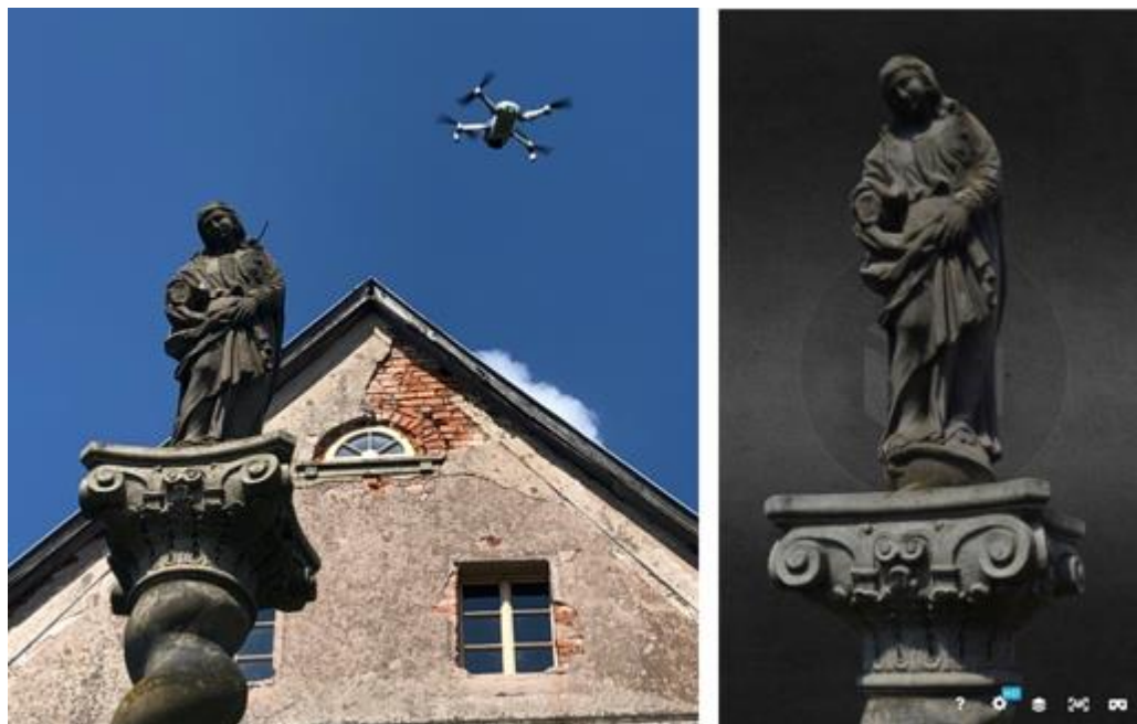
Fig. 1. On the left, a drone taking pictures of the Virgin Mary statue in Hejtmánkovice. On the right, the finished 3D model of the sculpture presented on the Sketchfab platform. You can view the 3D model of the statue of the Virgin Mary on Sketchfab at the following shortened link: https://skfb.ly/oqxDr
