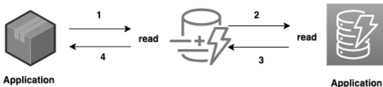
Fig. 2. Read-through cache algorithm
