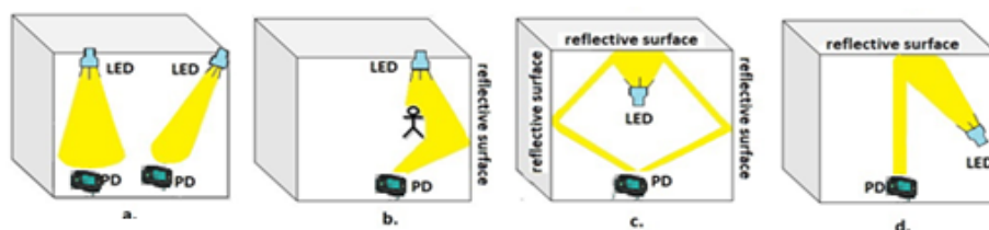
Fig. 3. a. Direct Line of Side (LoS) link, b. NLoS link, c. Diffuse link d. Quasi-diffuse link
